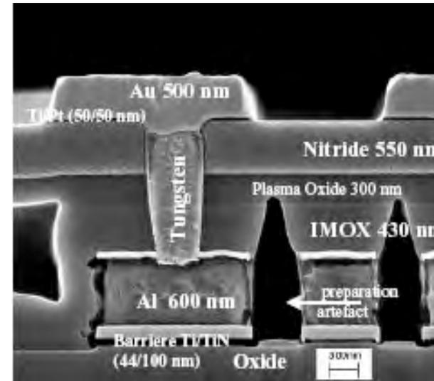
Additional process steps to expose and contact gold sensor electrodes
